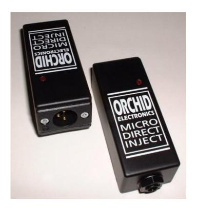
Housed in a strong aluminium die cast box 100 X 38 X 32 it has only a jack socket input for connection to the instrument and an XLR output to feed the microphone input of a mixing desk - which can be located many hundreds of metres away if necessary. It must receive Phantom Power from the mixer as it is an active design - a flush mounted red LED will indicate power present.
